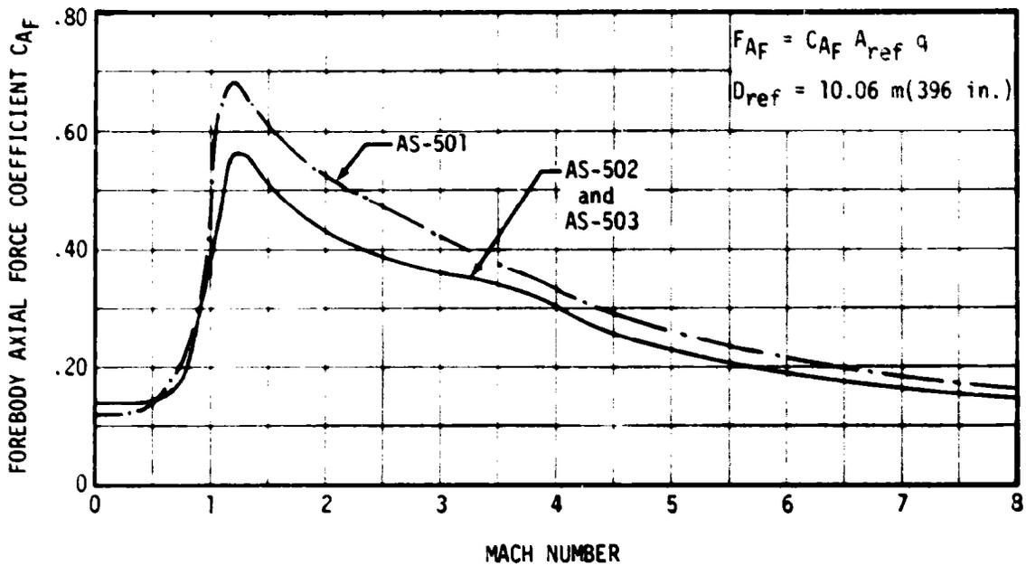
Figure 20-2. Forebody Axial Force Coefficient
